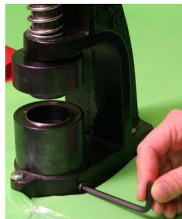
**5. Setting Grommets:** Ensure that fingers and other body parts are away from the setting dies. With a slow, firm, even motion pull the lever down as far as it will go, then apply additional pressure for a few seconds. Release the lever and remove the finished grommet assembly. Inspect the grommet on both sides to ensure that it was set properly. If required; return grommet assembly back onto the bottom die and repeat.
